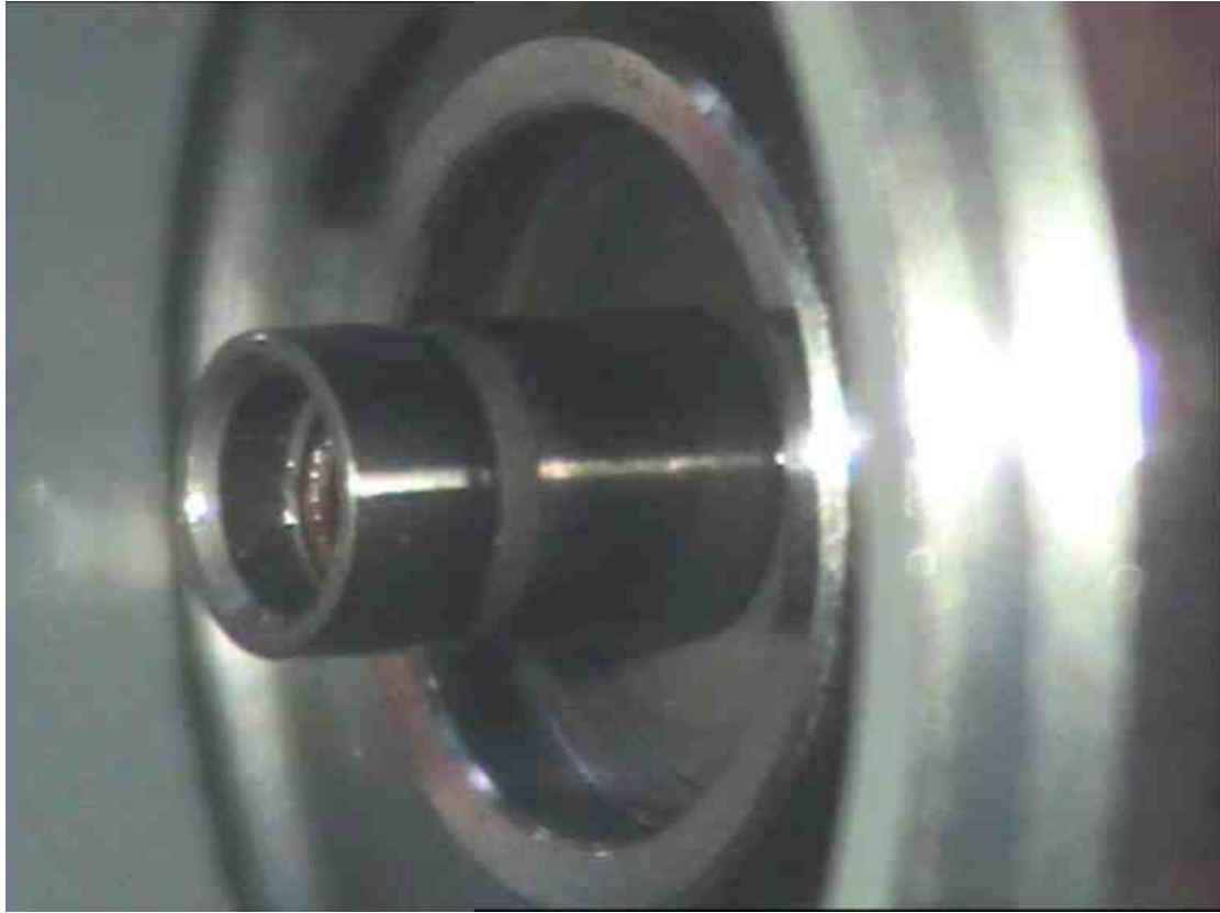
Above: Side view of the rotor, showing the (fluid) bearing surface.
