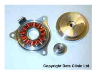
**Above:** Disassembly of the spindle motor from a seized Maxtor N40P series hard drive. The parts are (left to right): starter motor, fluid bearing, rotor
